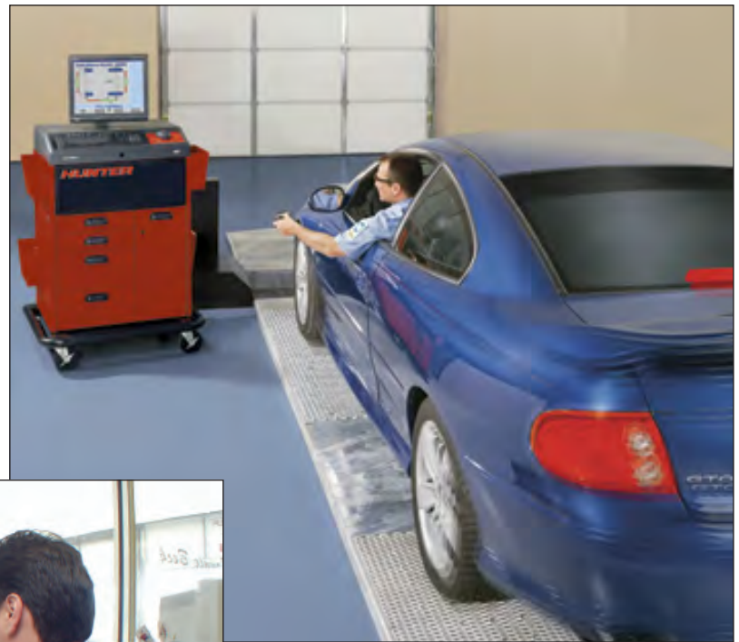
Computerized inspection equipment performs complete vehicle undercar inspections in three minutes or less.
